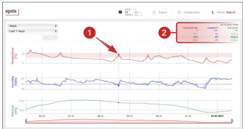
The lines displayed in full color show the logged average values. The lighter areas around the lines represent the minimum and maximum values recorded in the specific timeframe. The horizontal bars represent the limit values at which alerts are triggered. Their width corresponds to the specified dead band. The exact values for a specific time are displayed in the upper right corner (2) when you move the cursor along the graph (1).
