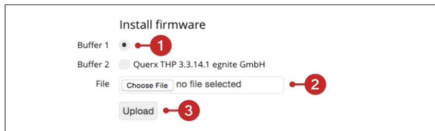
1. Select the *Buffer* in which you want to save the firmware image in the section *Install firmware*. You should choose either an empty buffer, or the one with the oldest firmware version.
