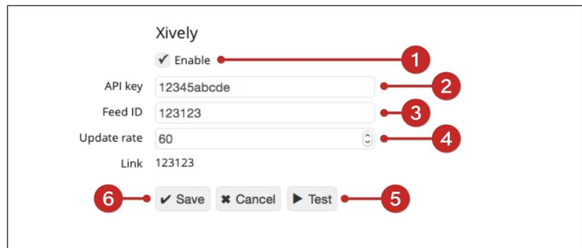
The screenshot shows the 'Xively' configuration section. It includes a checked 'Enable' checkbox (1), an 'API key' input field with '12345abcde' (2), a 'Feed ID' input field with '123123' (3), an 'Update rate' input field with '60' (4), and a 'Link' field with '123123'. At the bottom, there are 'Save' (6), 'Cancel', and 'Test' (5) buttons.
