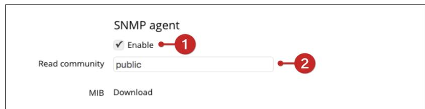
1. Activate SNMP by clicking the checkbox *Enable*.
