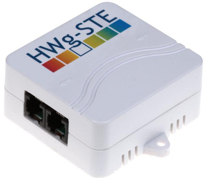
HWg-STE is a web thermometer with built-in web interface and SNMP support. It sends e-mail alerts if the temperature exceeds a specified limit.
