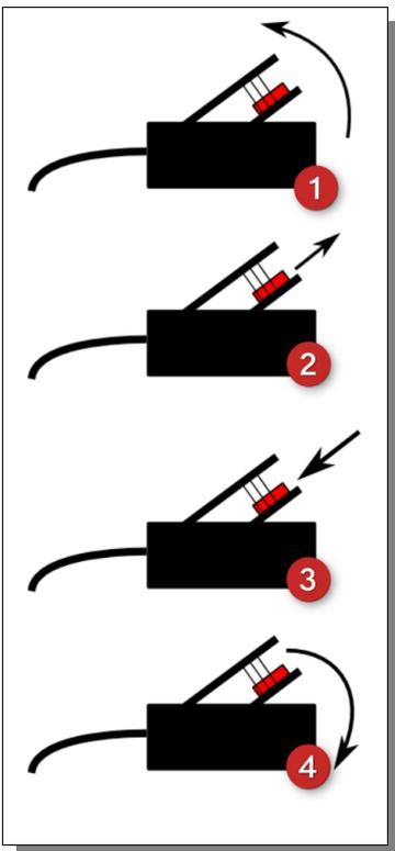
1. Carefully lift the circuit board up at the edge opposite the sensor cable.
