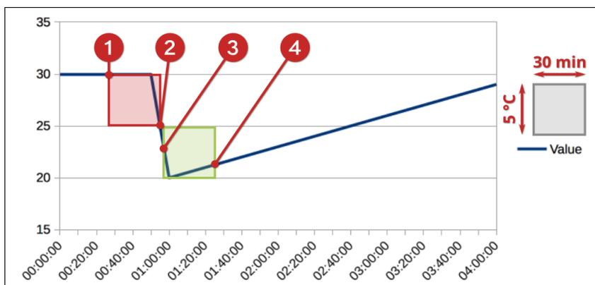
The diagram depicted above shows the way Querx reacts when a window is opened. The maximal rate at which the
