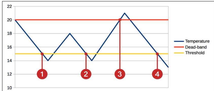
The minimum temperature is set to **15°C** in the example depicted above. The dead-band is set to **5°C**.
