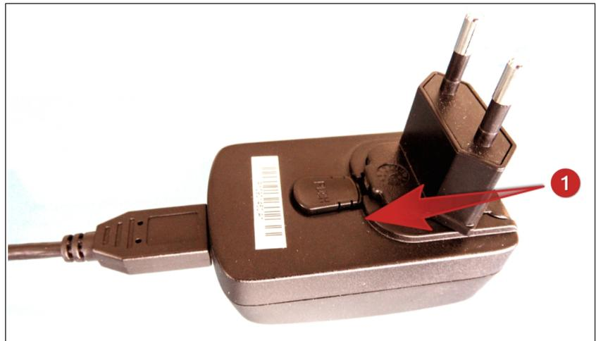
1. Prepare the power adapter by inserting the plug that is used in your country into the guide rail. An audible click indicates that the connection has been made.
