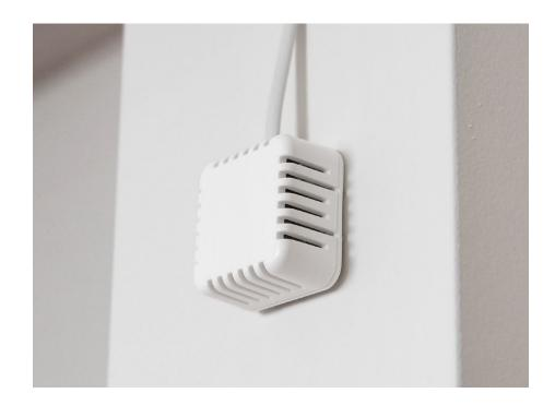
Two types of indoor sensor with 1-Wire RJ11 interface. Indoor sensors
