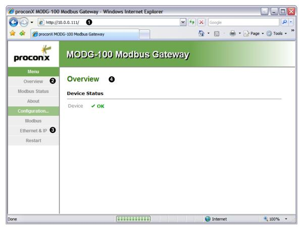
Figure 5.1: Device management and configuration via the web browser
