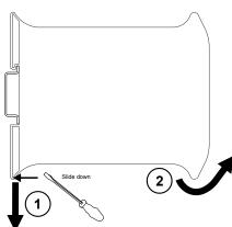
To remove the *MODG-100* from the DIN rail, use a screw driver as a lever by inserting it in the small slot of the red hook and push the red hook downwards. Then remove the unit from the rail by raising the bottom front edge of the enclosure.
