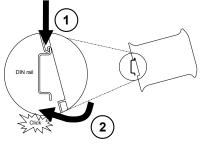
To mount the unit on a DIN rail, slot the top part of the *MODG-100* into the upper guide of the rail and lower the enclosure until the bottom of the red hook clicks into place.
