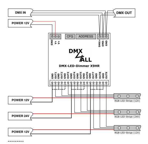
Must be connected direct from the power supply. Depends on the current for the LED-Stripes.
