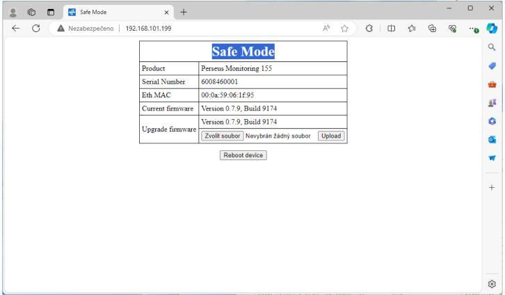
Factory Reset - Press the button, apply the power and wait for the Alam/Status LED to turn off. Releasing the button while the LED is flashing will ensure that the application is booted up with the current configuration.
