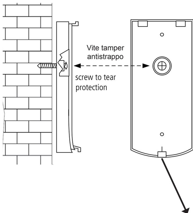
To open, use a flathead screwdriver into the slot and push
